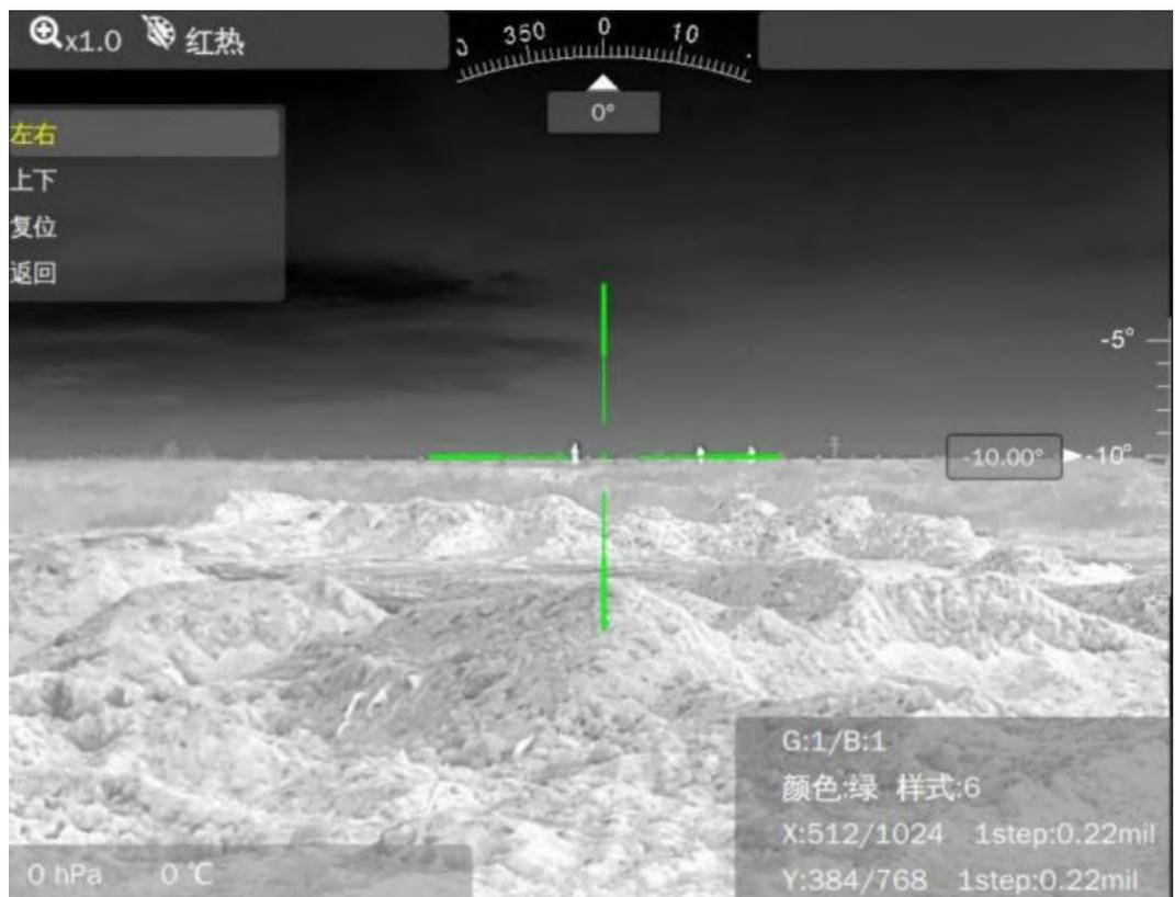
Figure 14 Gun calibration interface
